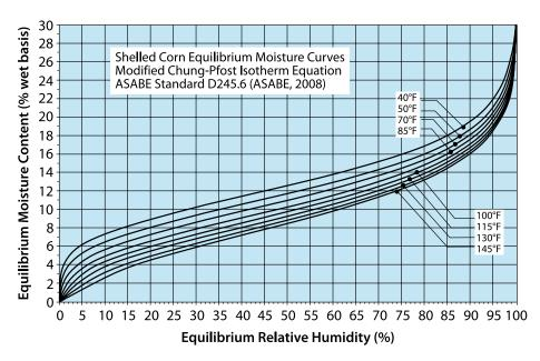
Figure 3. Equilibrium moisture content of shelled corn with air of various relative humidity and temperature.
