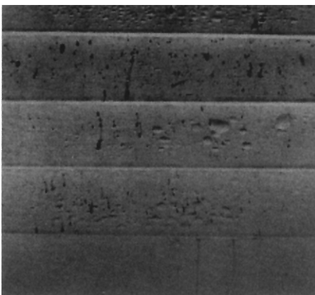
Figure 1. Moisture blistering and peeling.
