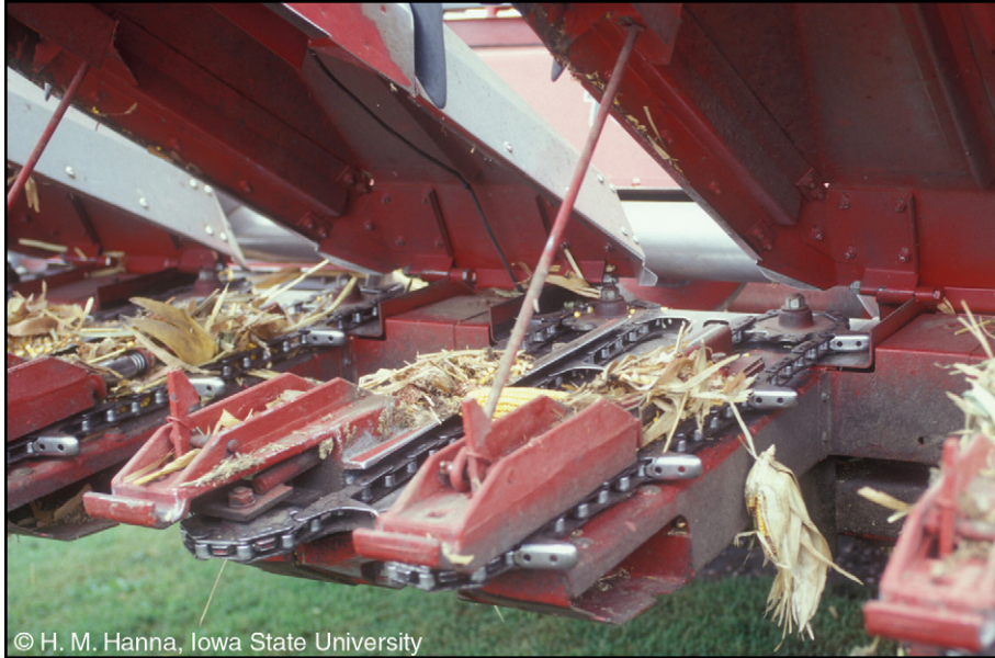
Figure 8. Corn residue underneath shields on cornhead
