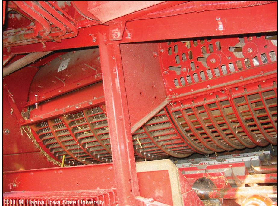
Figure 12. Wire concave area that wraps around the rotor
