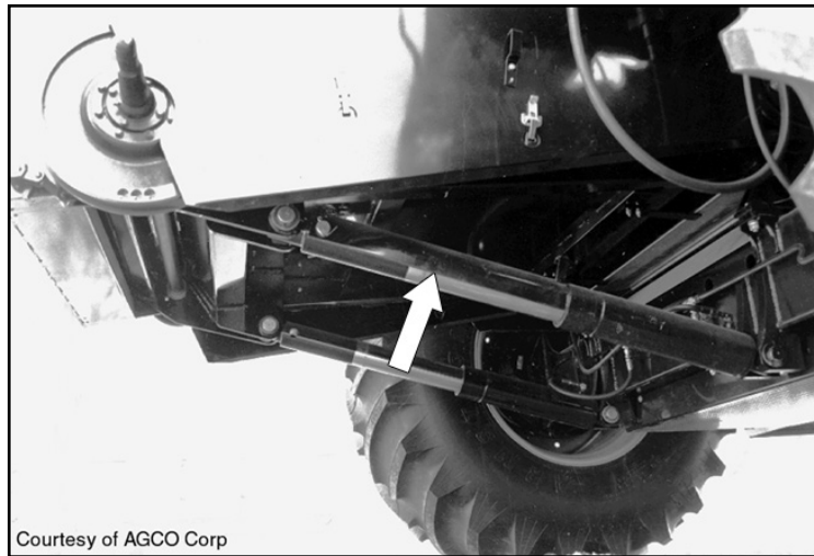
Figure 1. Feederhouse blocked up by cylinder stop
