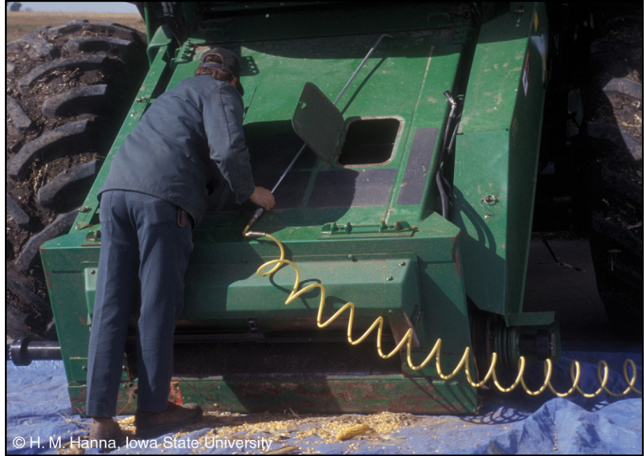
Figure 10. Inspecting feederhouse through top access doors
