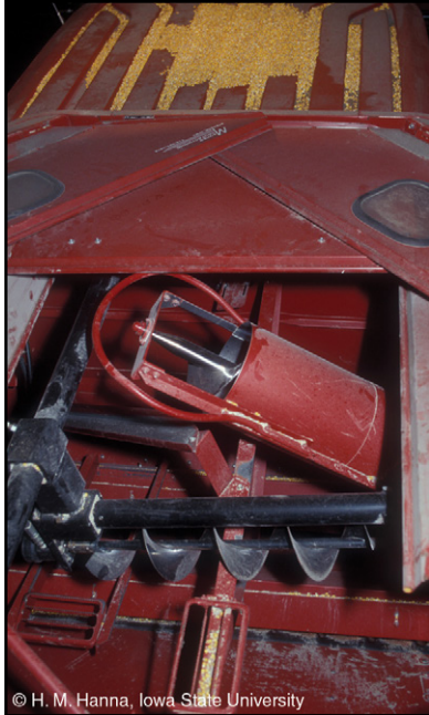
Figure 20. Augers in the grain tank. Note corn spilled on the cab roof in background.
