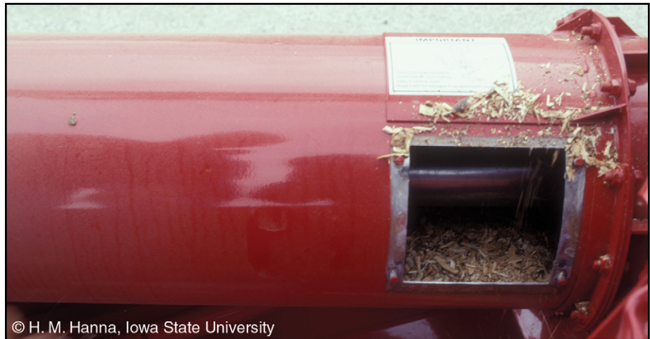
Figure 23. Access panel removed on unloading auger housing
