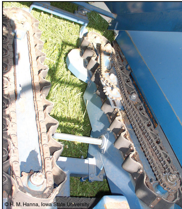
Figure 31. Gathering mechanisms on the head exposed after the center shield was lifted
