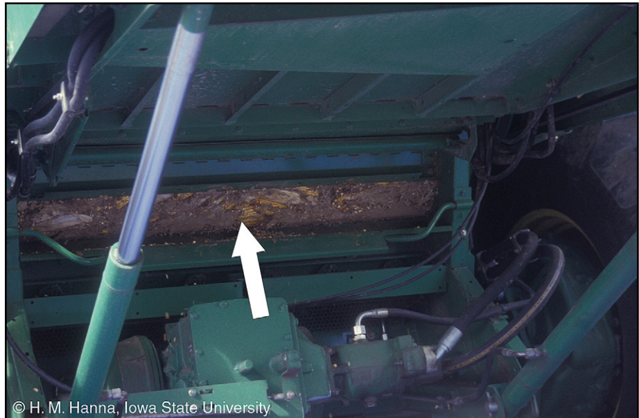
Figure 11. Rock trap opened underneath feederhouse (corn residue visible)
