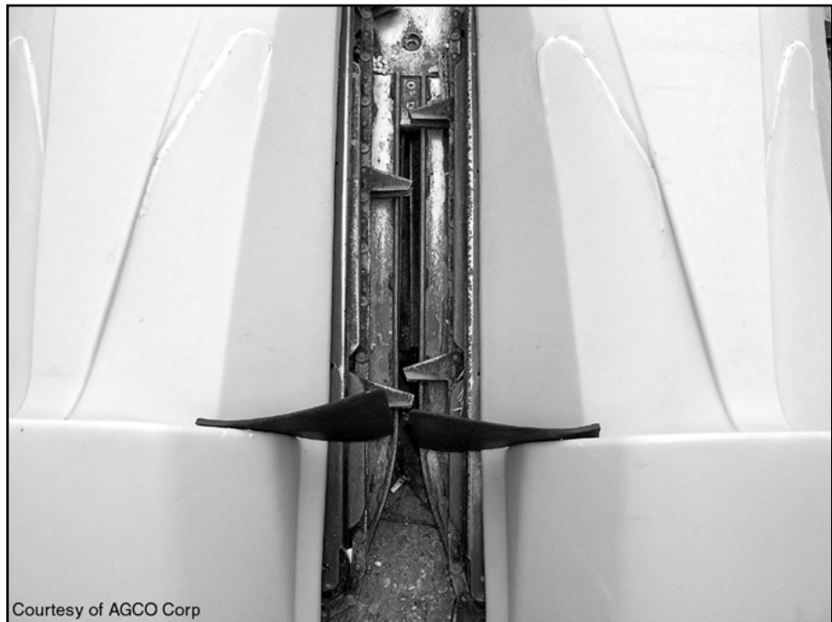
Figure 7. Shielded snapping rolls on cornhead row unit
