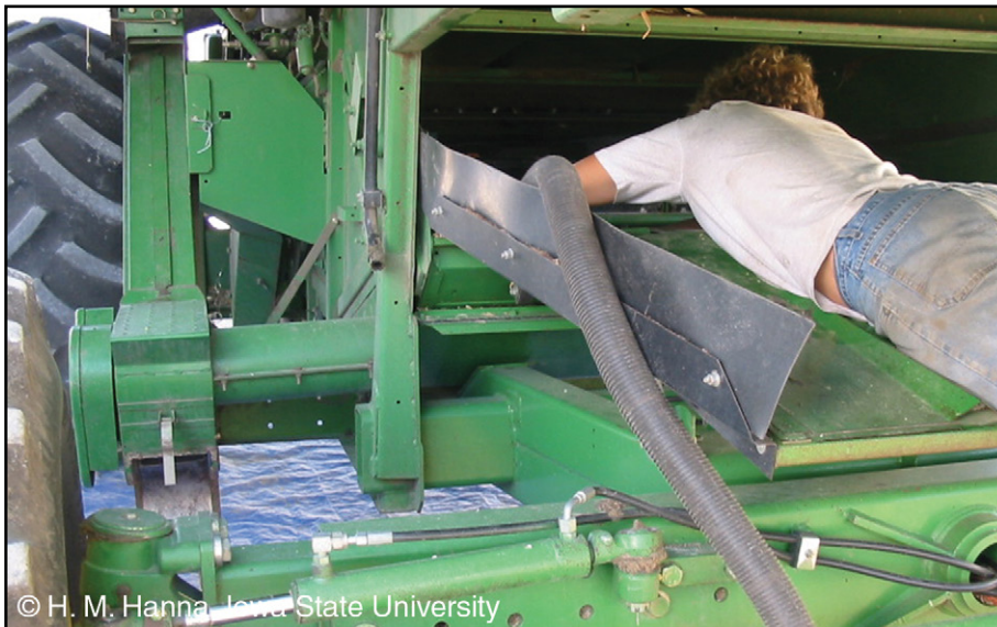
Figure 18. Vacuuming in the rear of the cleaning shoe
