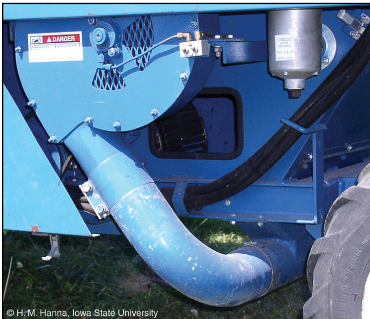
Figure 35. Pneumatic air tube as it bends from fan to collection area underneath combine
