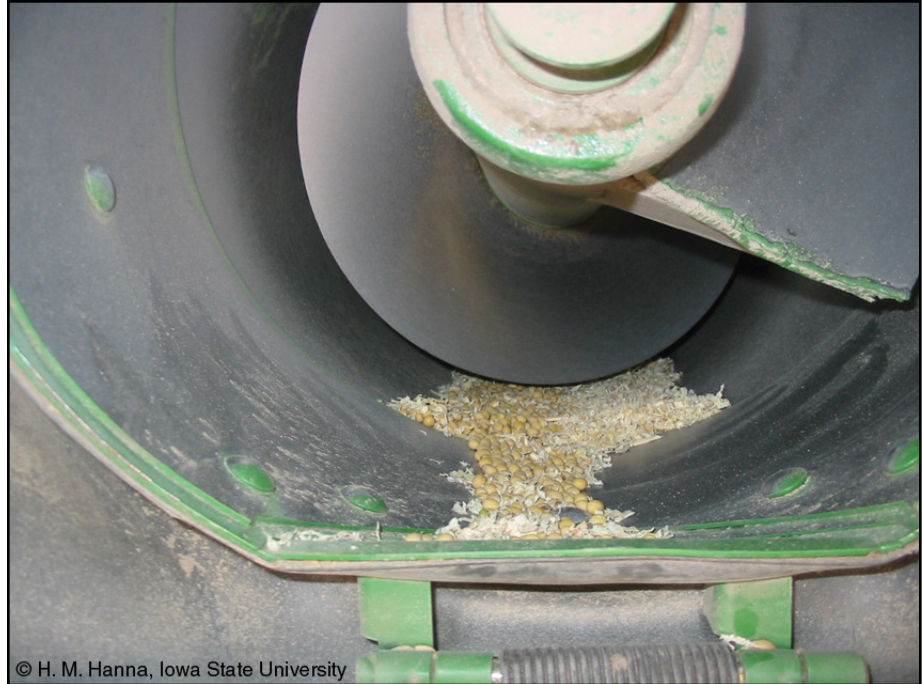
Figure 22. Exit of unloading auger with spring-loaded door folded down
