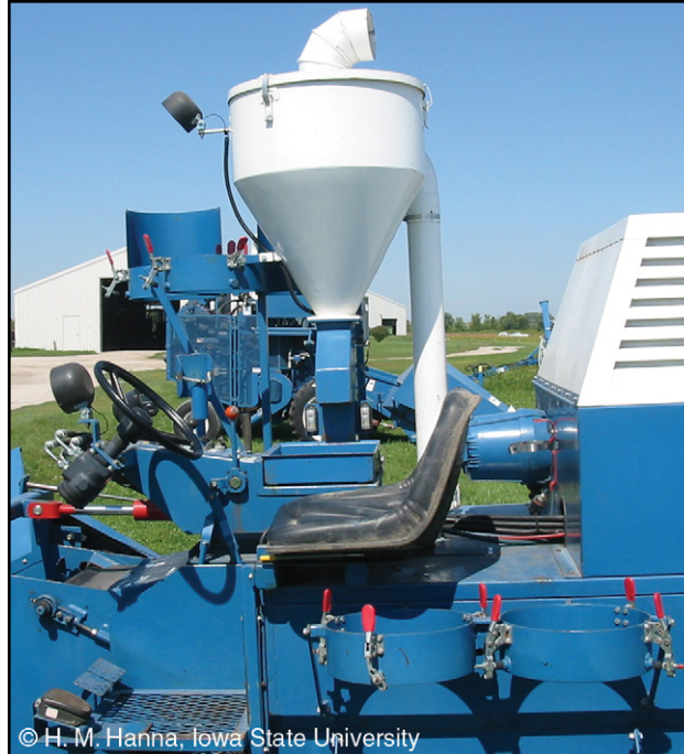
Figure 36. Operator's station just ahead of the engine compartment
