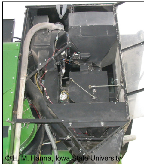
Figure 29. Modification on commercial combine (right of the cab) to weigh grain samples
