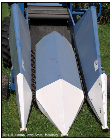
Figure 30. Two-row head on a small combine used for soybean harvest
