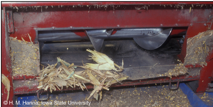
Figure 9. Opening into rear of cornhead showing cross-auger
