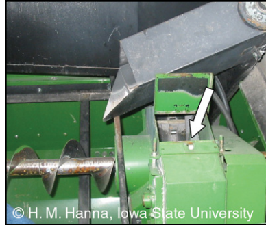
Figure 28. Top of a grain elevator with the access door open to expose the diverter flap to redirect grain to an in-cab weighing hopper
