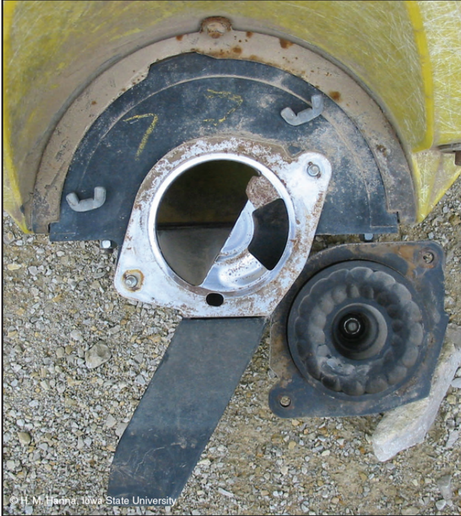
Figure 22. Seed cup meter after cover is removed
