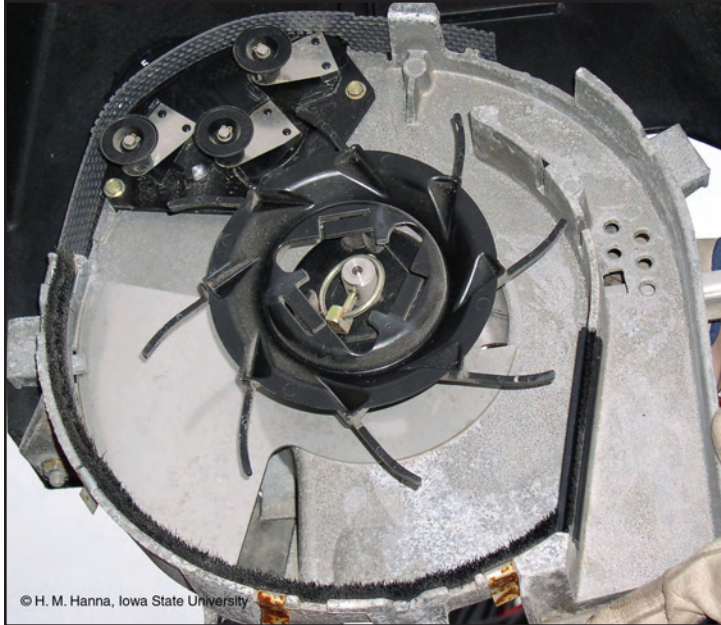
Figure 16. Exposed seed meter after seed plate has been removed
