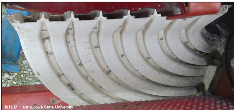
Figure 30. Seed exits into air tubes underneath seed drum
