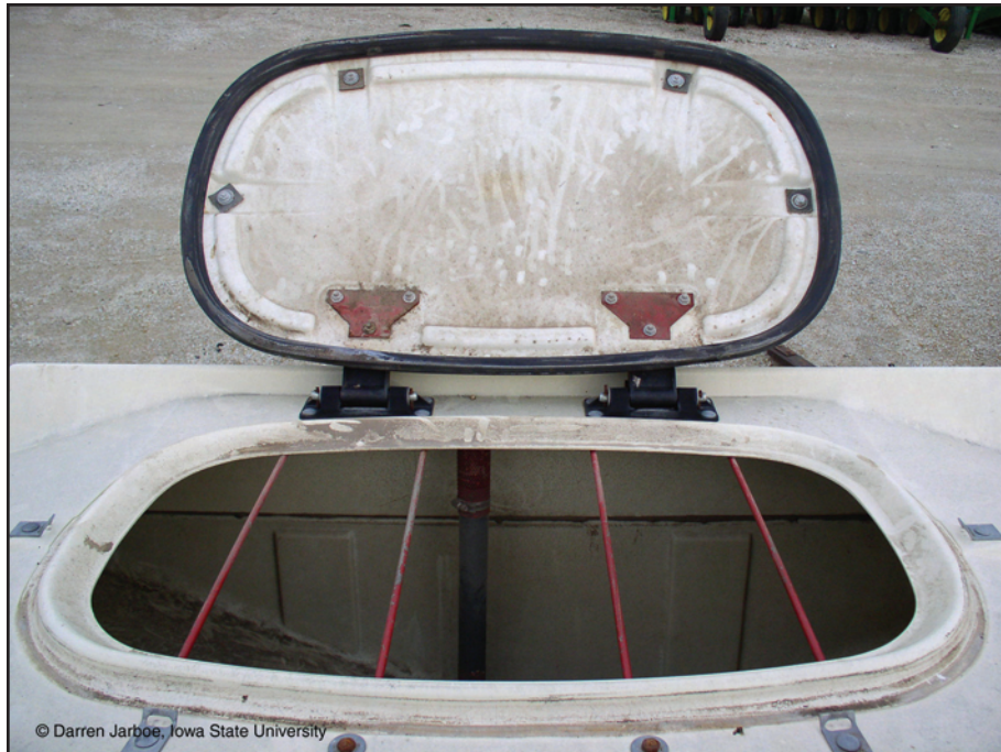
Figure 25. Seed hopper with open lid (note gasket seal)
