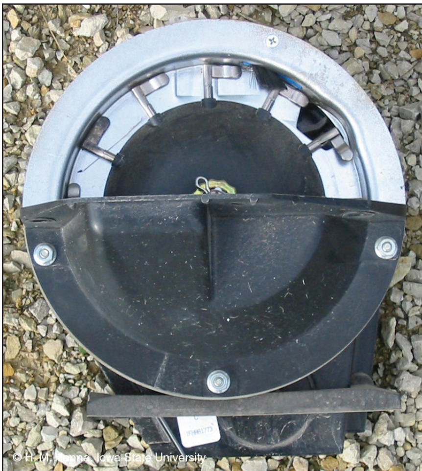
Figure 20. Cover over finger-type seed meter mechanism
