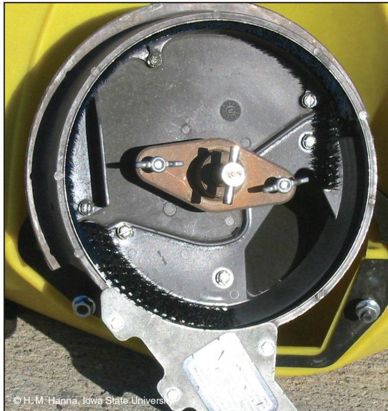
Figure 24. Exposed brush meter opened after seed plate is removed
