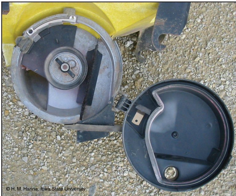
Figure 13. Door open showing vacuum seed meter with brush and gasket seal
