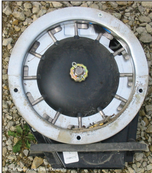
Figure 17. Finger-type metering mechanism with cover exposed
