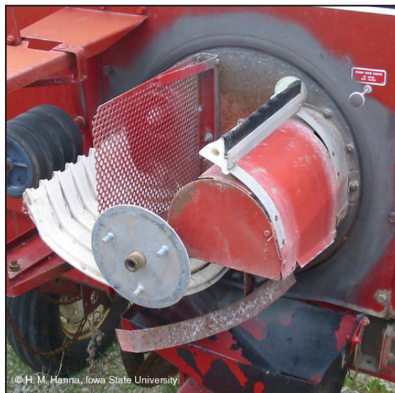
Figure 27. Seed metering area after removal of seed drum
