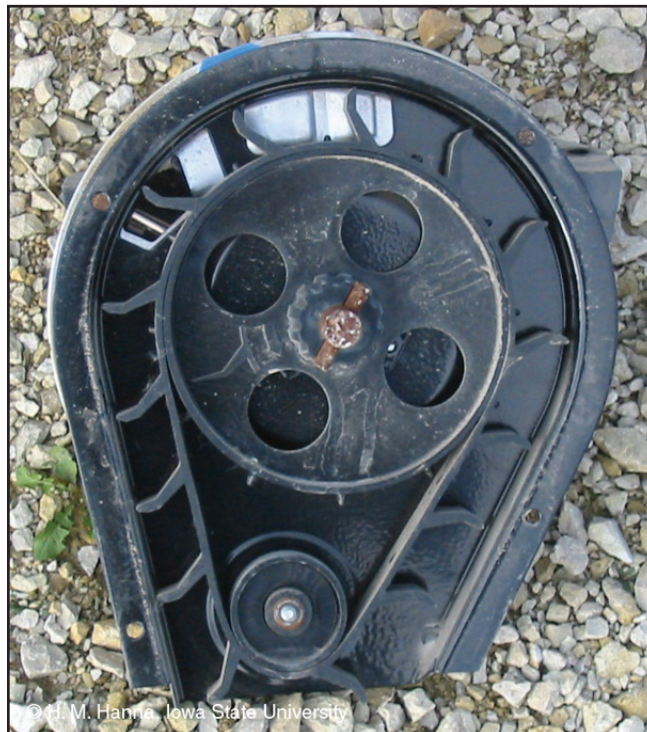
Figure 18. Belt conveyor used to deliver seed from meter to seed drop tube
