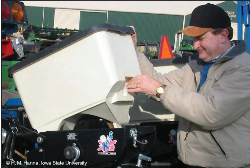
Figure 19. Removing hopper/meter assembly after first disengaging seed drive
