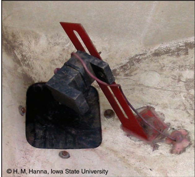
Figure 28. Seed sensor in bottom of seed hopper
