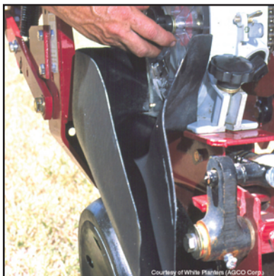
Figure 34. Seed funnel used on side of meter on newer models
