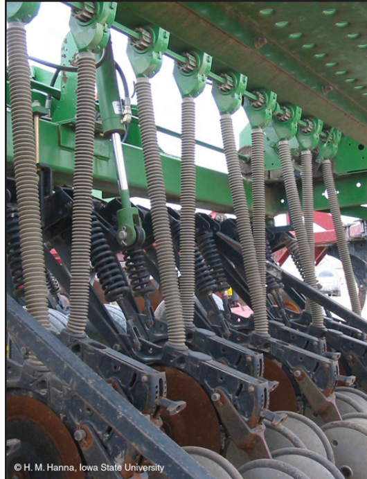
Figure 10. Seed drop tube on grain drill between meter and opener
