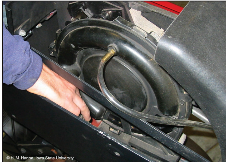
Figure 14. Disconnecting vacuum hose
