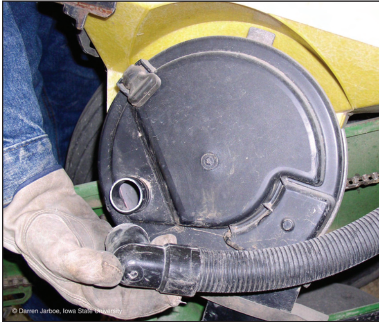
Figure 12. Disconnecting vacuum hose from hopper assembly
