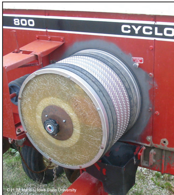
Figure 26. Seed drum on side of central hopper
