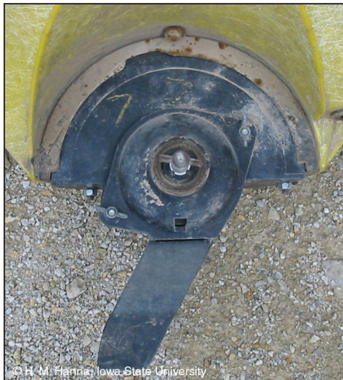
Figure 21. Seed cup meter with cover
