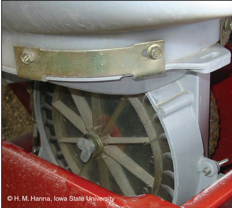
Figure 32. Seed plate fastened by center attachment bolt
