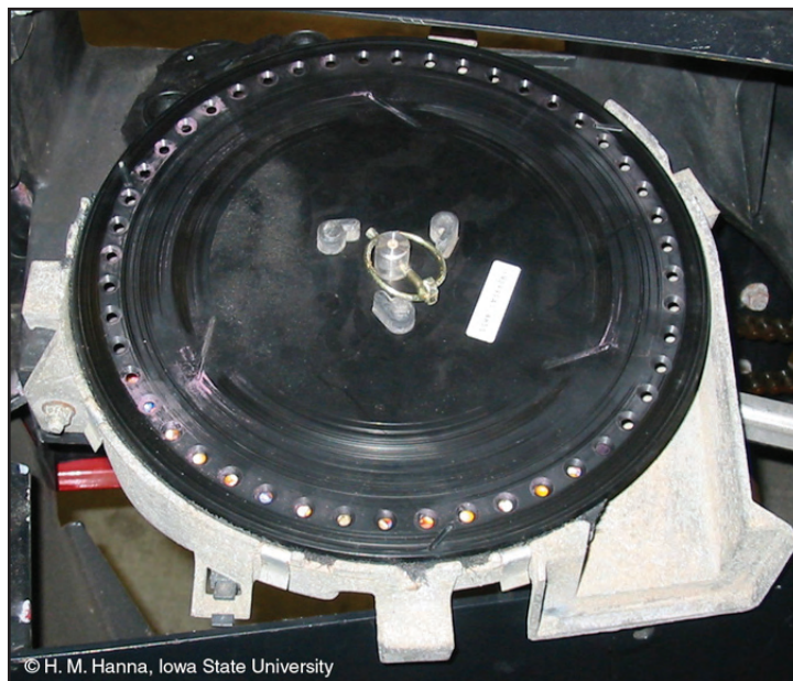
Figure 15. Seed meter with seed plate
