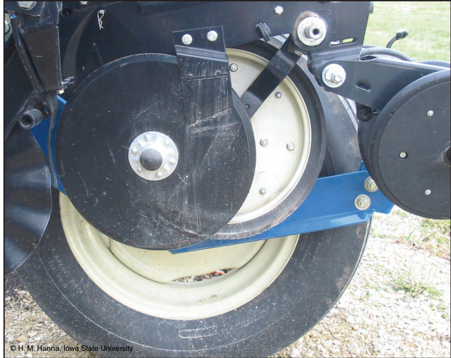
Figure 38. Depth wheel removed exposing disc on one side of double-disc seed opener
