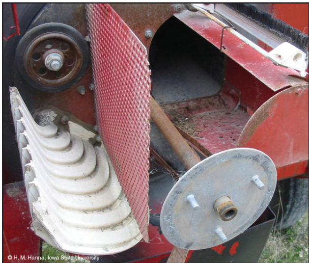
Figure 29. Air intake flange underneath seed drum
