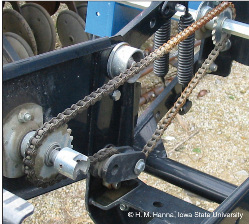
Figure 1. The chain transmission drive on planter is a possible pinch point
