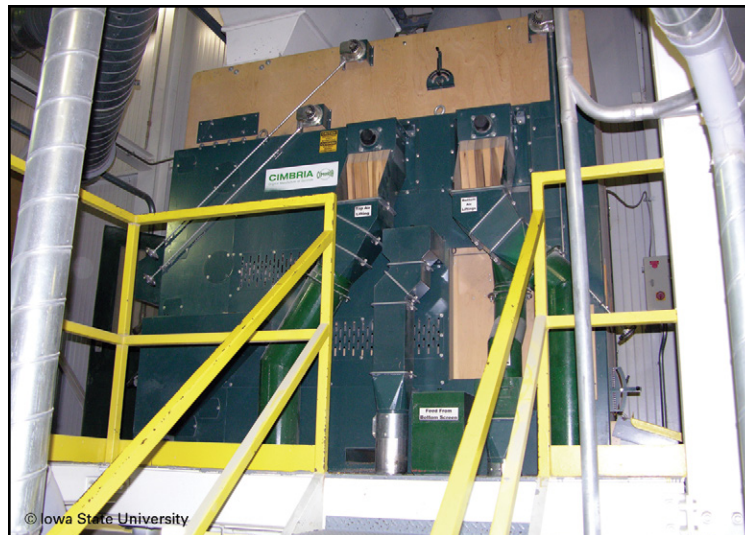
Figure 5. An oscillating sieve machine in a processing plant
