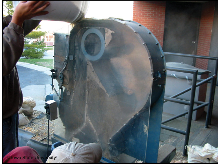
Figure 7. Laboratory-sized aspirator with plexiglass side. Centrifugal fan within upper-left corner of aspirator sucks (and separates) lighter material from grain falling past it.
