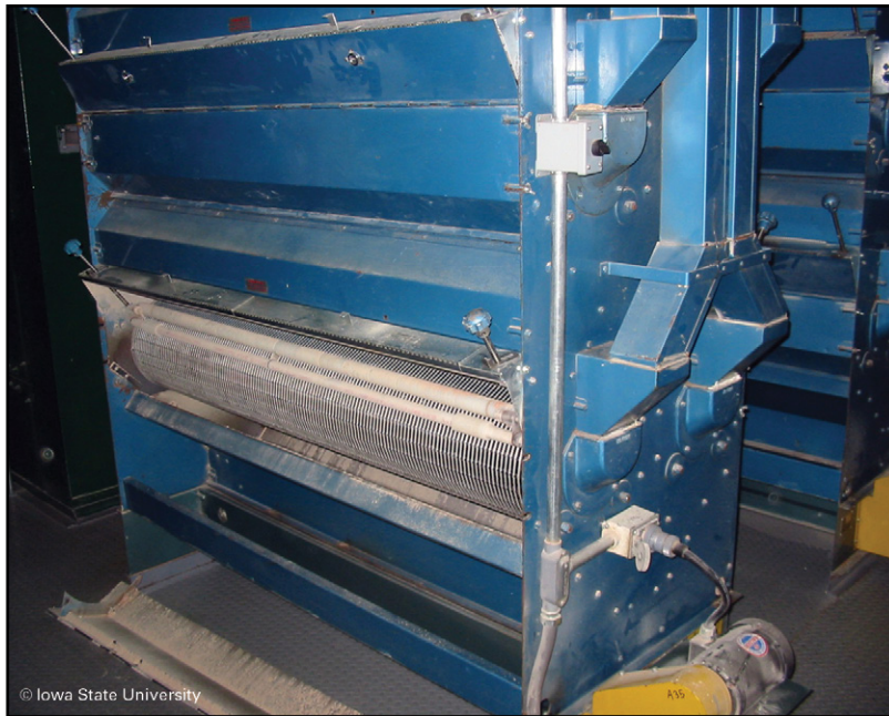
Figure 14. Cylindrical screen separator with a cover removed to expose cylindrical screen (note feed tubes on right side of machine)
