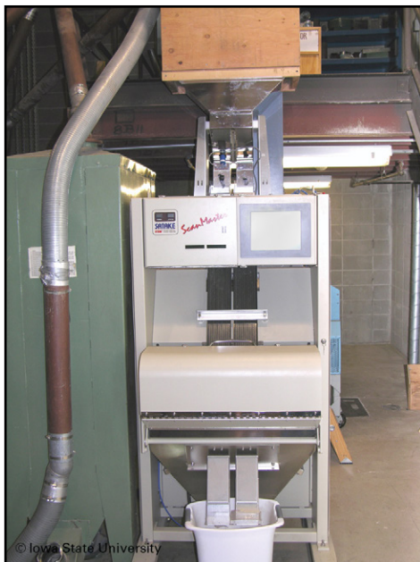
Figure 17. Color sorter (overhead feed hopper supplying single-seed depth flow down lower black channels past color sensor into separate flow streams at bottom)
