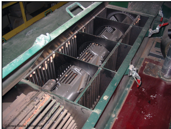
Figure 16. Stationary sheller with rotor surrounded by open wire concave (note bits of cob wedged between concave bars in upper left and general cob "dust" atop concave in lower left foreground)
