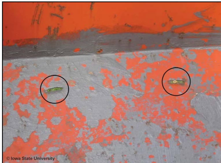
Figure 5. Holes in grain box (just below seam between sidewall and hopper bottom)
