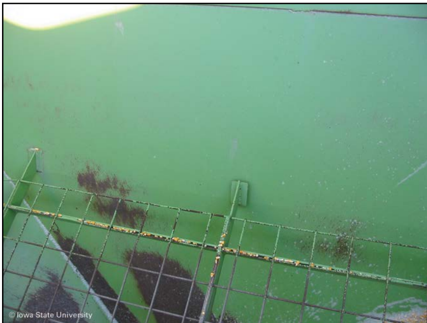
Figure 22. Safety grate over auger intake in bottom of grain cart
