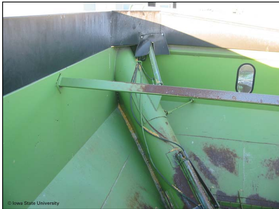
Figure 20. Auger housing inside box on grain cart (note cross support in foreground)
