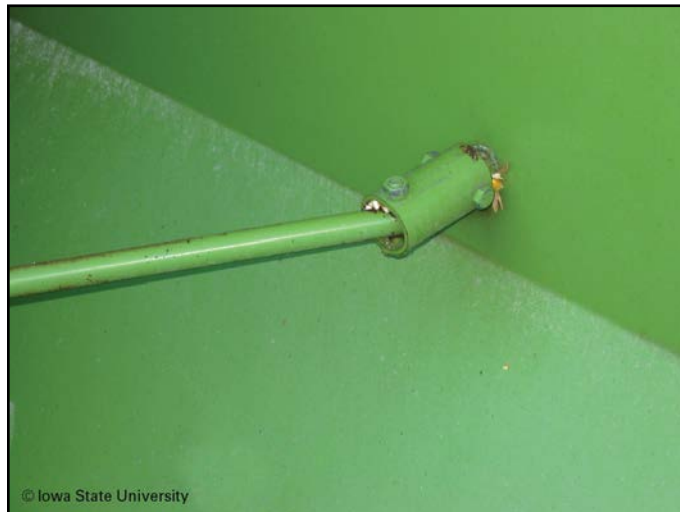
Figure 9. Cross-support attached to grain box wall
