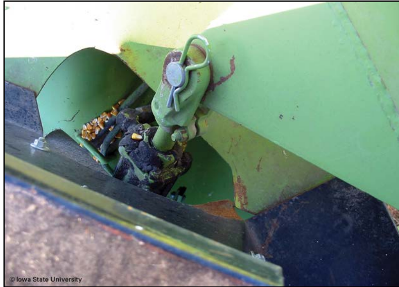
Figure 13. Grain on horizontal exterior surface and exposed grease near hydraulic ram
