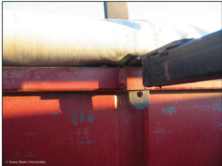
Figure 18. Rolled-up tarp sitting on top edge of truck grain box next to a cross-support (note grain between tarp and grain box edge; if open, end of hollow tube should also be inspected)
