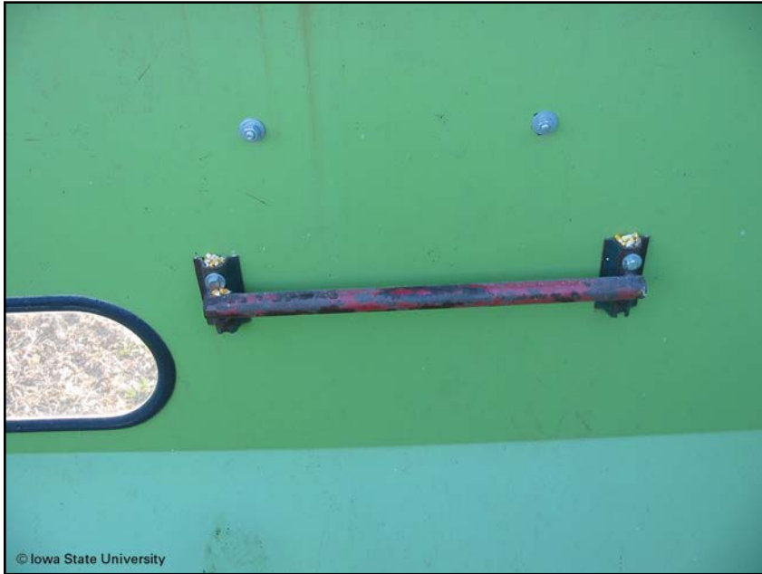
Figure 21. Interior access step in grain cart (note window with gasket on left)
