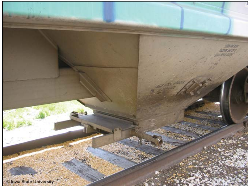
Figure 24. Sliding door at bottom of hopper
