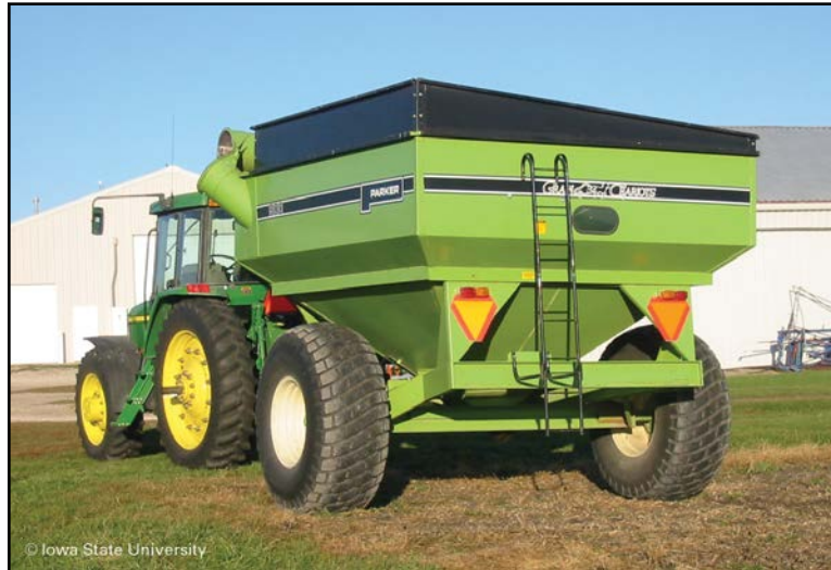
Figure 4. Single-axle grain cart (folding point of unloading auger just visible at upper left corner of grain box)
