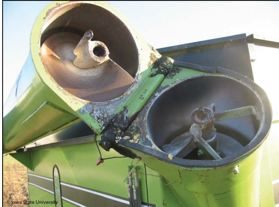
Figure 19. Exposed folding point with auger folded in transport position
