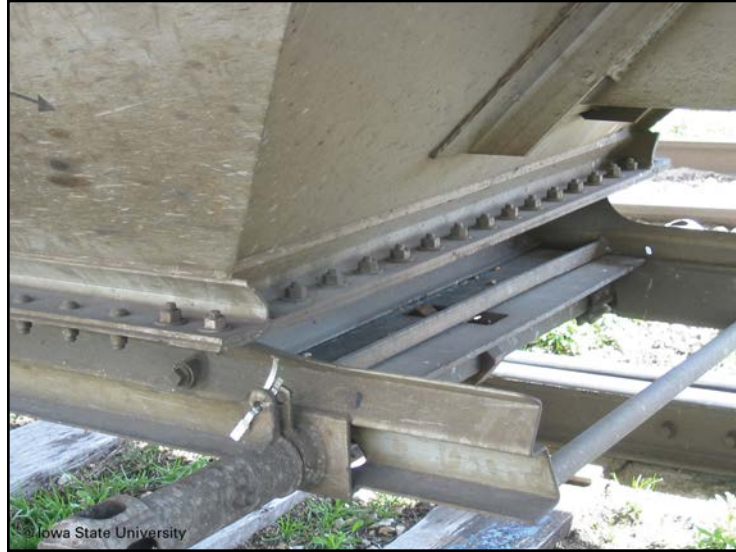
Figure 31. Retracting side of bottom door (note grain kernels atop door near opening edge)
