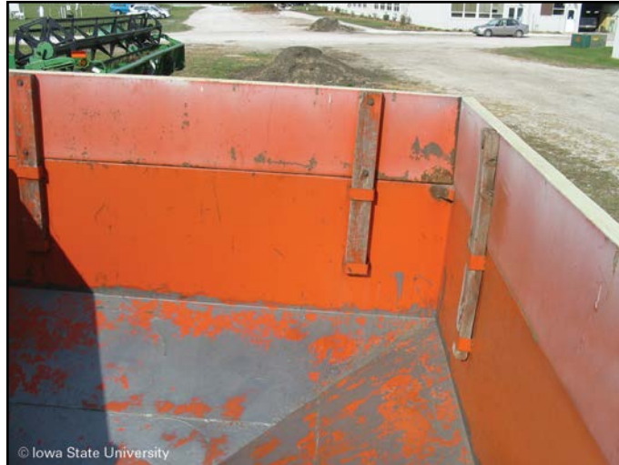
Figure 8. Extensions to extend sidewall height at the top of the grain box
