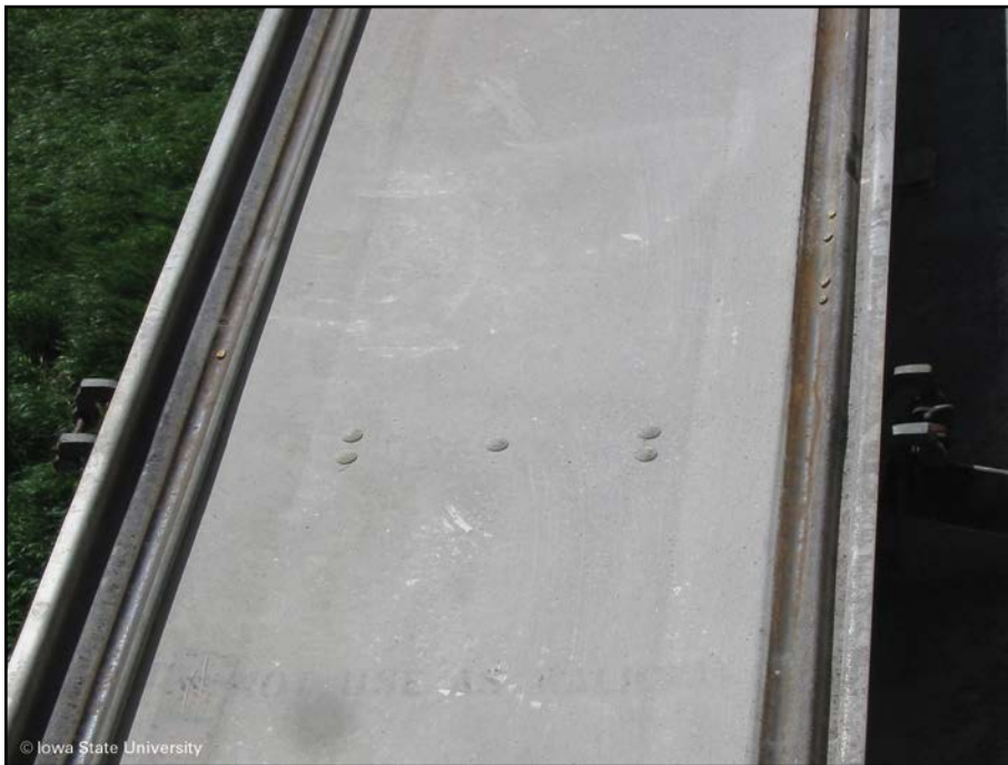
Figure 26. Gasketed seal inside either side of opened top hatch (note grain kernels on gasket)
