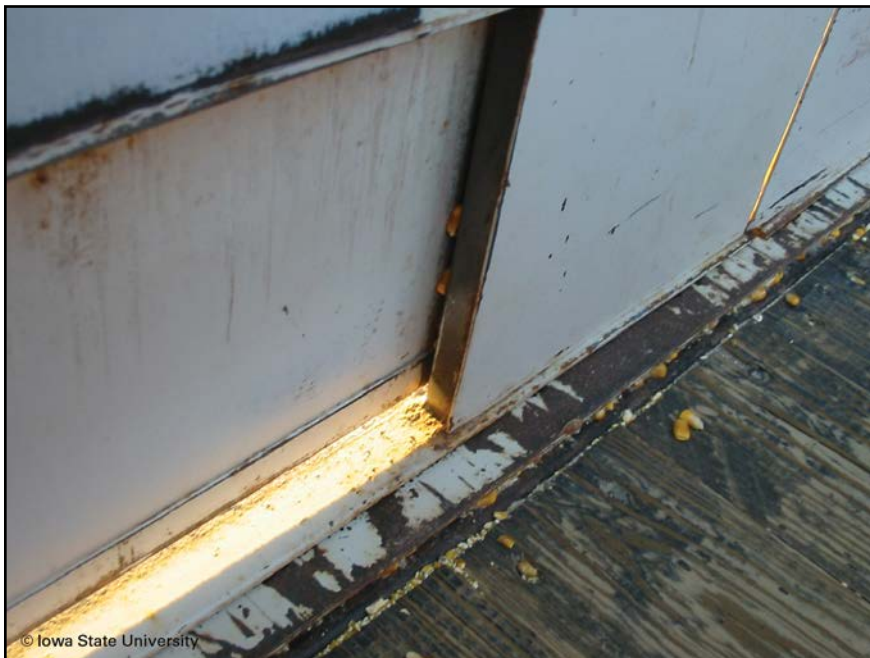
Figure 12. Grain caught in slide track along edge of retractable door (note also grain lodged in seam on box floor next to doorway)
