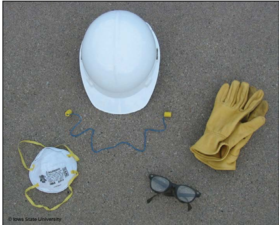
Figure 6. Personal protective equipment including two-strap dust mask, ear plugs, hard hat, safety glasses (folded side shields not visible), and gloves
