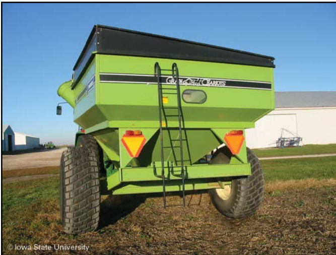
Figure 2. Grain box with hopper-shaped bottom to funnel grain to unloading auger entry (hidden by lower frame) at bottom center of grain cart
