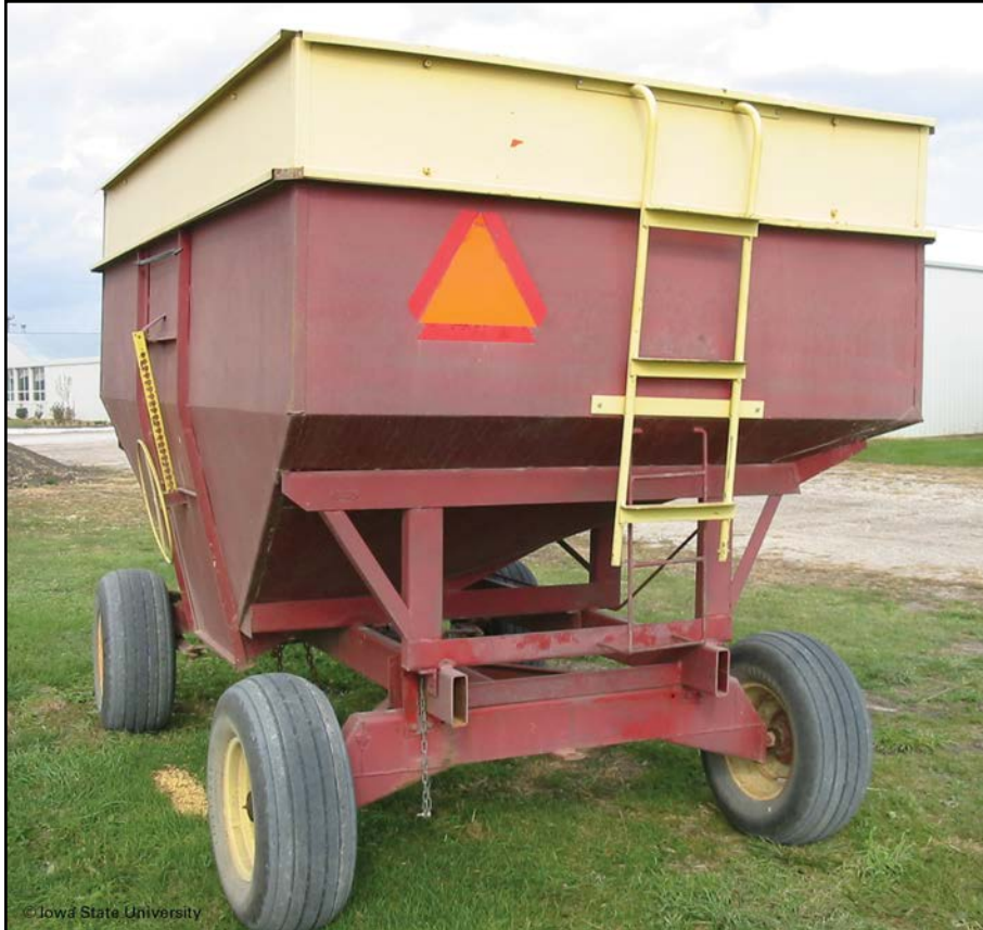
Figure 7. Wagon with hopper bottom for unloading by gravity through retractable door on left side (note exterior access ladder)
