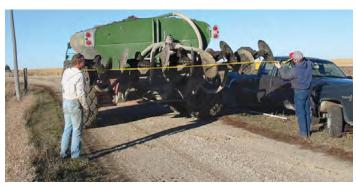
Figure 3. Measuring the application swath width.
