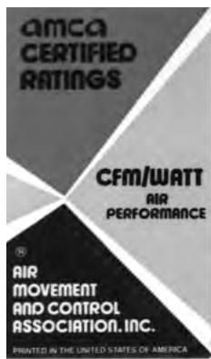
Figure 3. This label indicates that the fan has been tested by the Air Movement and Control Association (AMCA)
