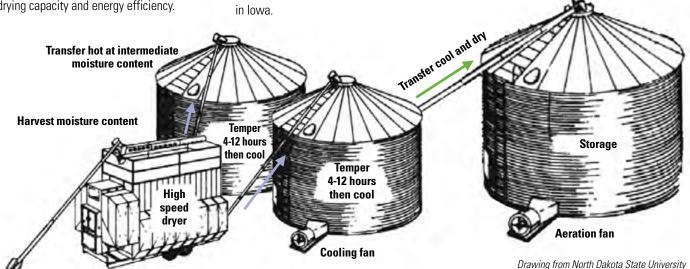
**Dryeration example:** high-temperature dryer system with two tempering bins. Tempering bins are filled in alternating order, making sure hot grain has at least 4 hours of time to temper before exposure to cooling air. After tempering and cooling, transfer grain to storage bin.
