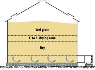
Figure 1. Low-temperature grain drying
