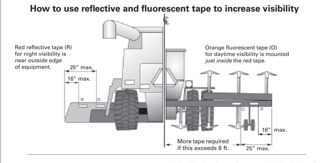
This shows correct placement of tape on a combine (left) and a tractor towing a field cultivator (right), with a slow-moving vehicle emblem in the center. Equipment
