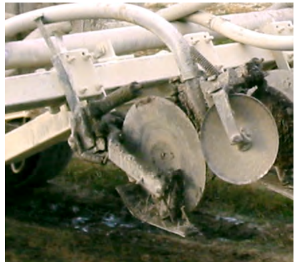
Figure 3. Slot injected manure applicator.
