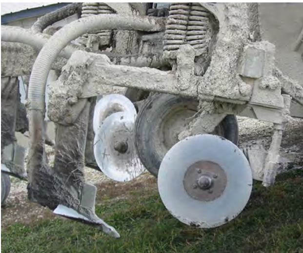
Figure 2. Shovel incorporated manure applicator.
