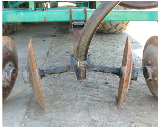
Figure 1. Disc-covered manure applicator.
