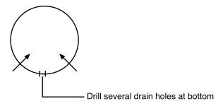
Figure 1. Drill holes in lower quarter of tube.
