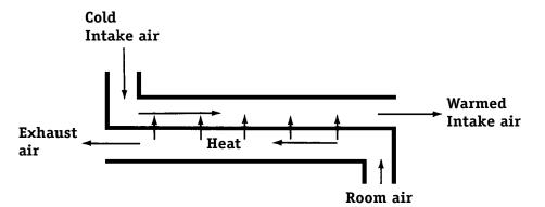
Figure 3. How a Heat Exchanger Works
