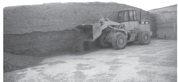
Figure 9b. Removing a uniform slice with a bucket.
