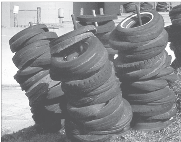
Figure 13. Split tires stacked vertically for easy access and to minimize problems with rodents.
