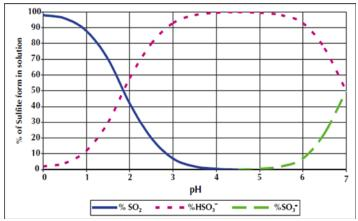
Figure 1. Percentage of forms of  $SO_2$ , molecular ( $SO_2$ ), bisulfite ( $HSO_3^{-2}$ ), and sulfite ( $SO_3^{-2}$ ) in wine over pH 0-7. Adapted from: Practical Winery & Vineyard, 2014.
