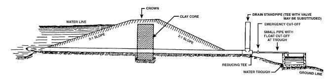
Cross section of dam showing water trough & drain lines. Turn drain pipe down to lower water level or drain pond.
