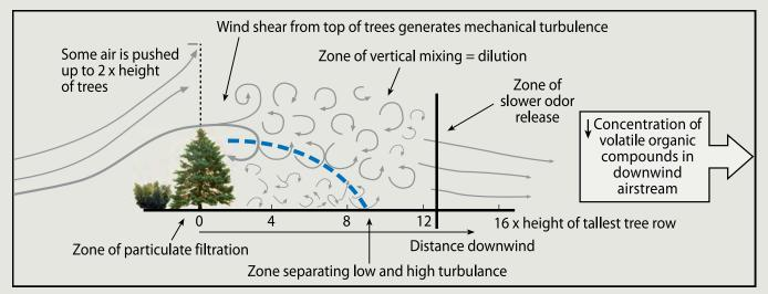
Fig. 2. Diagram displays generalized shelterbelt odor mitigation dynamics featuring increased turbulence, vertical air mixing, and articulate/odor filtration.
