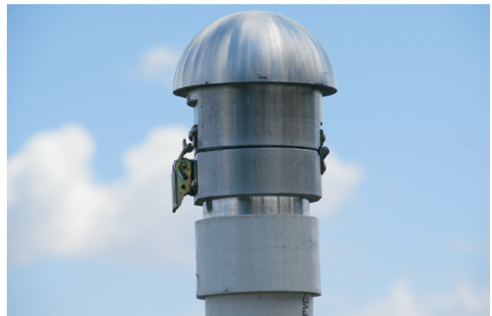
Close up of the head of the particulate matter sampler
