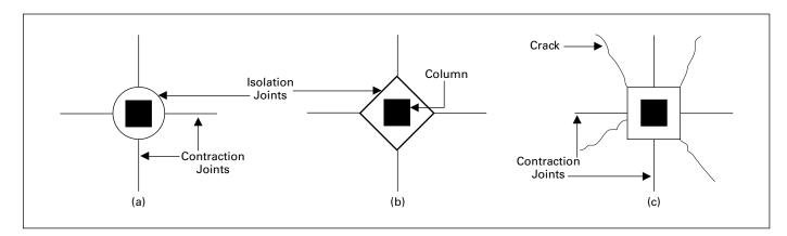
Figure 1. Isolation joints around columns can be circular (a) or square (b). If no isolation joints are used around columns or if the corners of the isolation joint do not meet contraction joints, radial cracking (c) can occur.
