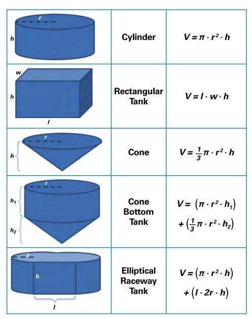
**Figure 1.** Formulas for calculating the volume of some commonly used tank shapes.
