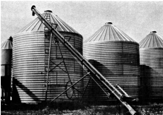
Fig 3. A portable auger can be used to fill bulk storage.
