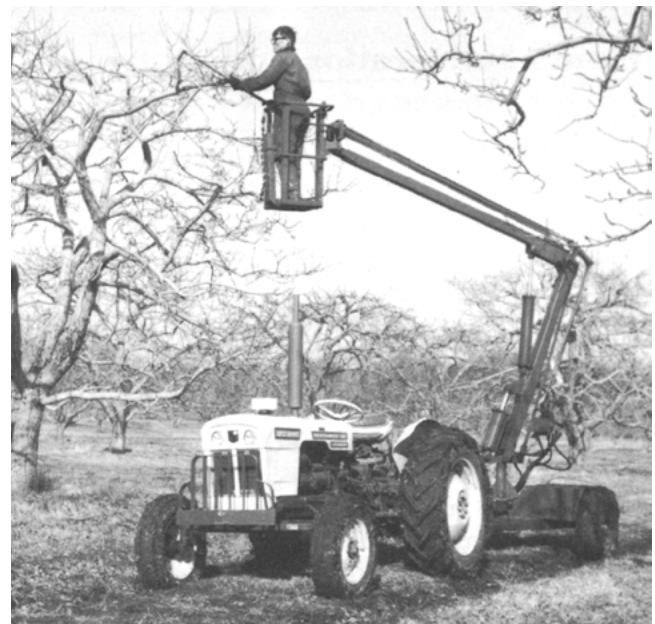
Figure 2. Hydraulically controlled towers and pruning equipment increase worker efficiency. Equipment operates from the tractor hydraulic system or is available as a self-propelled unit.
