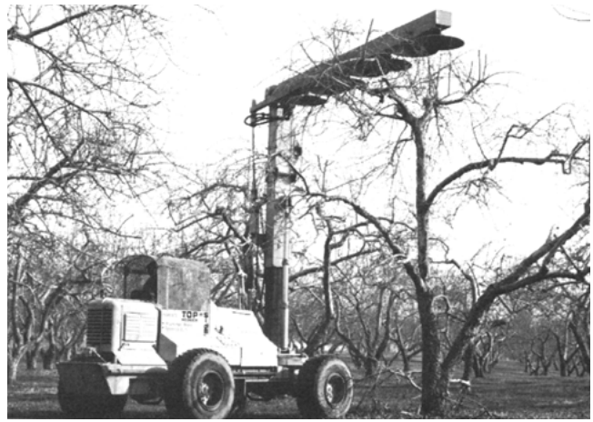
Figure 5. Hedging and topping machines of various types are being used to some extent to do bulk pruning in large orchards.
