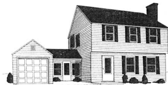
Two-story house with horizontal siding
