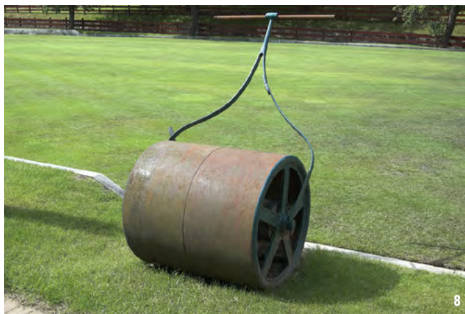
Figure 4. Rolling the newly laid sod will remove air pockets under the sod strips and increase rooting by pressing the roots firmly into the soil.
