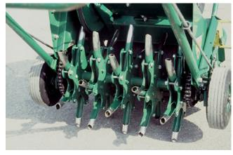
Figure 3. A core aerating machine removes soil plugs and spreads them on the lawn.
