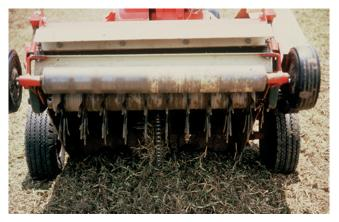
Figure 4. A vertical mower cuts through thatch and mixes soil into the existing thatch layer. Loose thatch deposited on the surface is hand raked for removal. The mower also can be used to prepare a good seedbed with channels for seed entry during lawn renovation.
