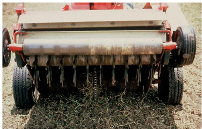
Figure 4. A vertical mower cuts through thatch and mixes soil into the existing thatch layer. Loose thatch deposited on the surface is hand raked for removal. The mower also can be used to prepare a good seedbed with channels for seed entry during lawn renovation.
