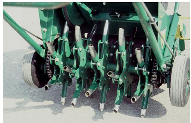
Figure 3. A core aerating machine removes soil plugs and spreads them on the lawn.
