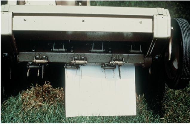
Figure 5. A spring-tined power rake can be used to remove about one quarter inch of thatch.
