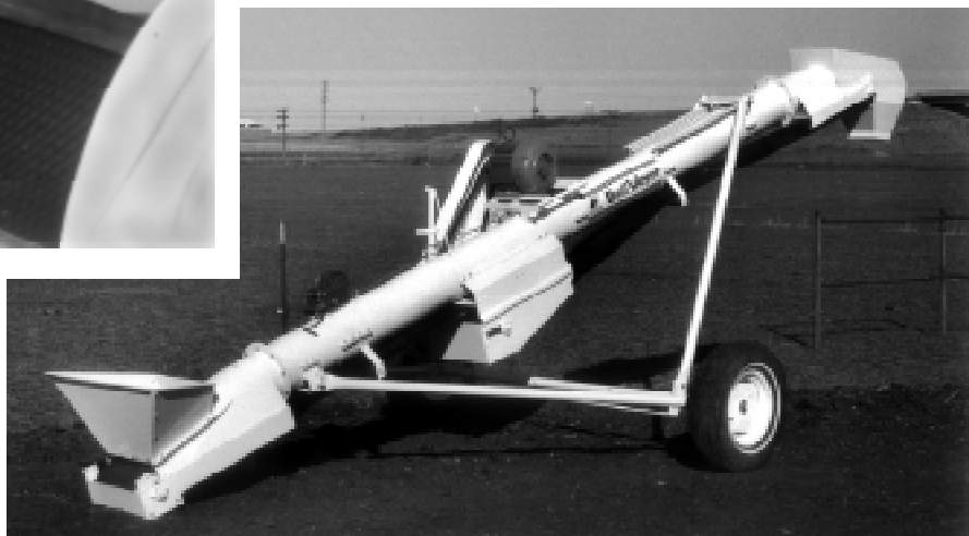
Figure 5. This conveyor has rubber flights attached to a rubber belt.
