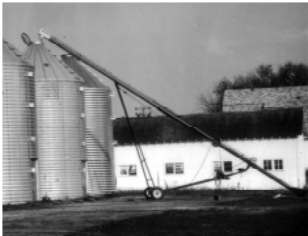
Figure 1. An auger is often used on the farm to fill bulk storage.
