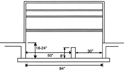
Figure 7. Gutter under raised crates.
