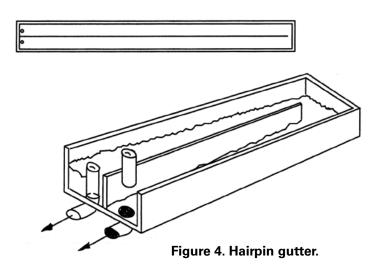
For a growing-finishing floor, make the gutter 24 to 36 inches deep and up to 100 feet long. In farrowing and nursery units, the gutter can be 18- to 24-inches deep and up to 50-60 feet long. Deeper gutters have been used, but may not be necessary.
