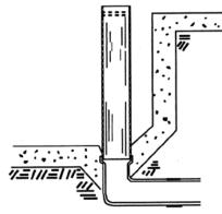
Figure 8b. PVC pipe for plug.
