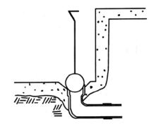
Figure 8c. Bowling ball for plug.
