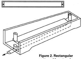
gutter with a step down.
