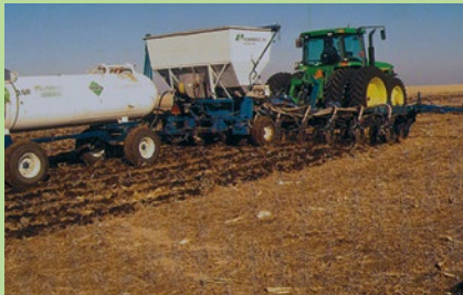
Fig. 2: Complete fall strip-tillage equipment system.
