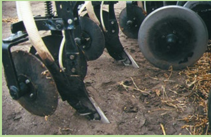
Fig. 1: Coulter, fertilizer injection knives, and covering disks on strip-tiller.
