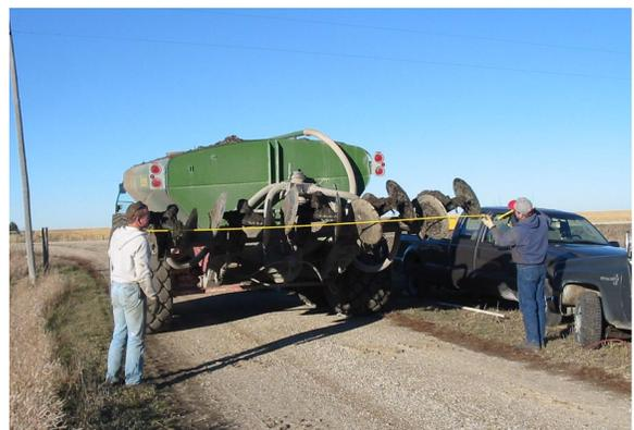
**Figure 3.** Measuring the application width.
