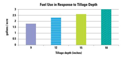
Figure 3. Diesel fuel used at different depths for subsoiler operation (Shinners, 1989).
