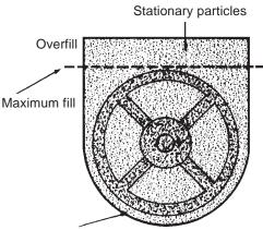
Stationary particles—nonmix zone (excessive clearance)
