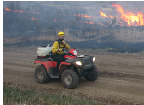
ATV mounted tank, pump, and hose reel for off-road fire suppression.
