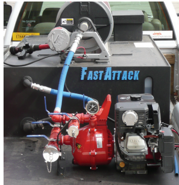
ATV mounted tank, pump, and hose reel for off-road fire suppression.
