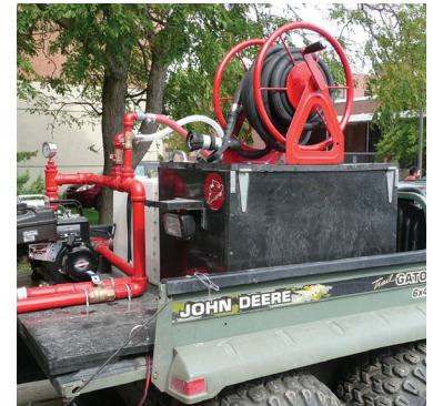
ATV mounted tank, pump, and hose reel for off-road fire suppression.
