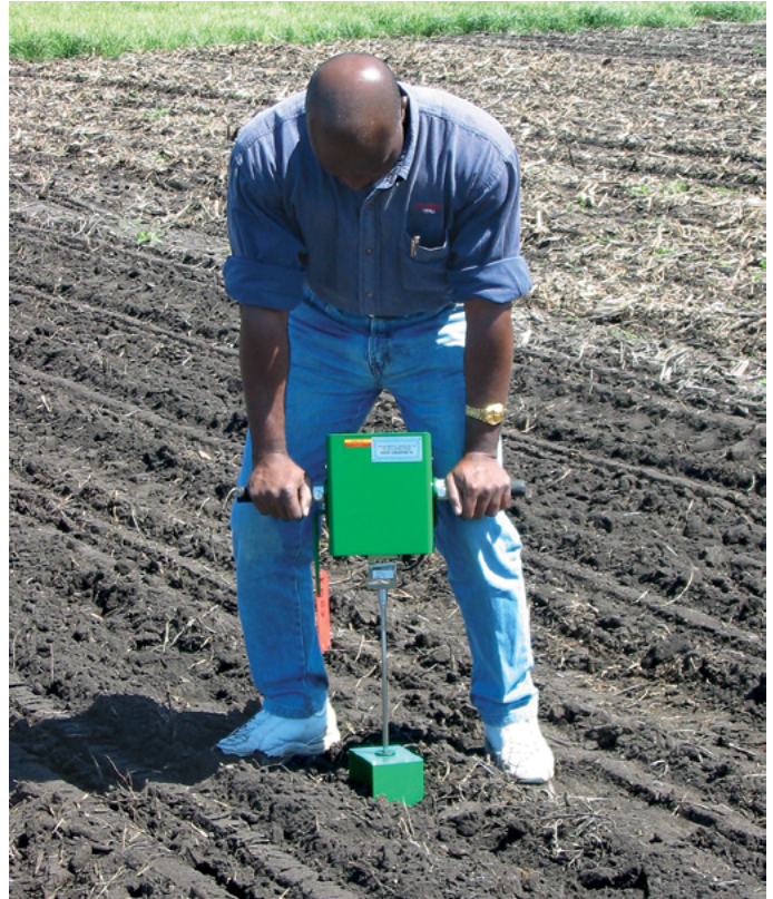
Measuring soil compaction
