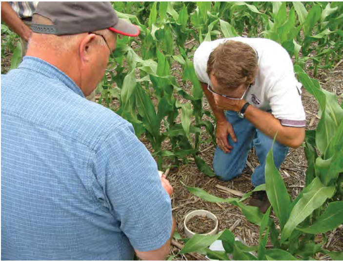
Demonstrating water infiltration in the field using a PVC ring
