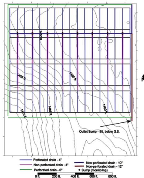
Figure 1. Schematic of plot layout and drainage monitoring system.
