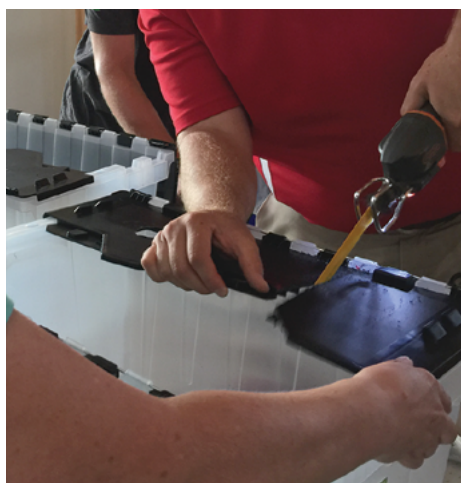
Figure 5. Cutting access door. (Photo credit: Shelly O’Neal, Linn County Extension)
