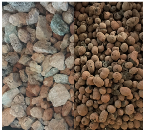
Figure 11. Growbed media. Lava rock (left) and pebbles (right). (Photo credit: Shelly O'Neal, Linn County Extension)
