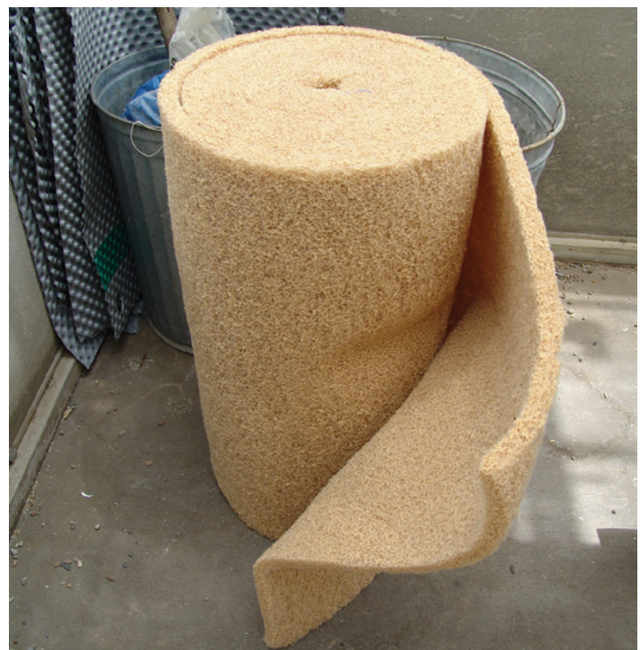
Figure 6. Solids filter pad material.
