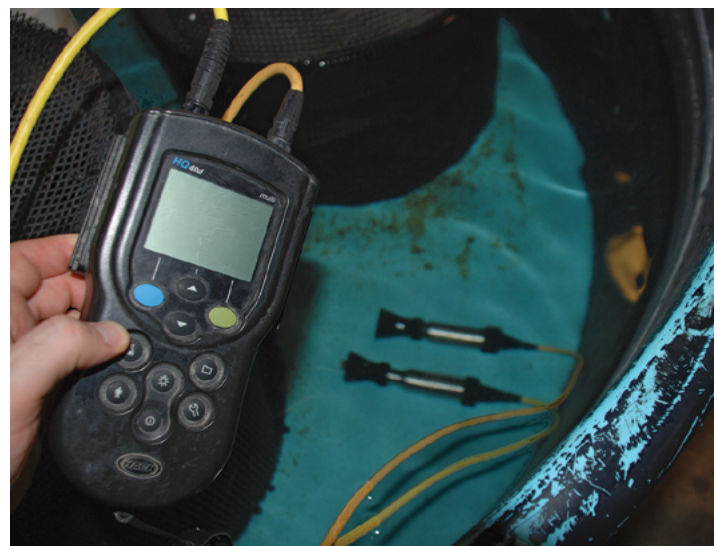
Figure 14. Measuring dissolved oxygen, pH and temperature with a water quality probe.
