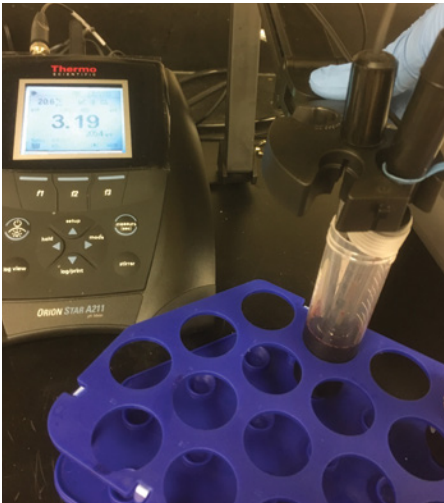
Measurement of pH on red wine sample.
