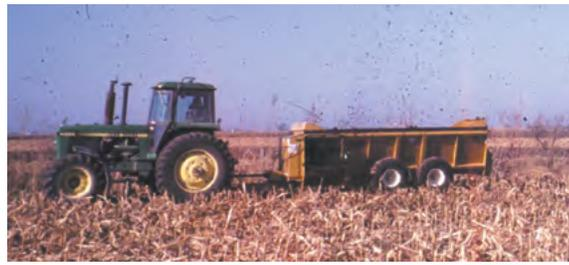
**Figure 5. Side-delivery spreader.**
