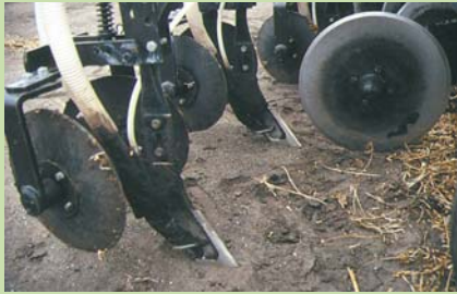
Fig. 1: Coulters, fertilizer injection knives, and covering disks on strip-tillager.
