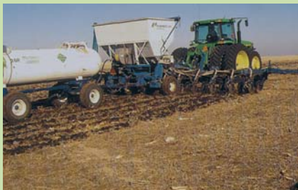
Fig. 2: Complete fall strip-tillage equipment system.
