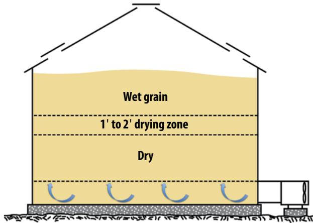
**Figure 1. Low-temperature grain drying**
