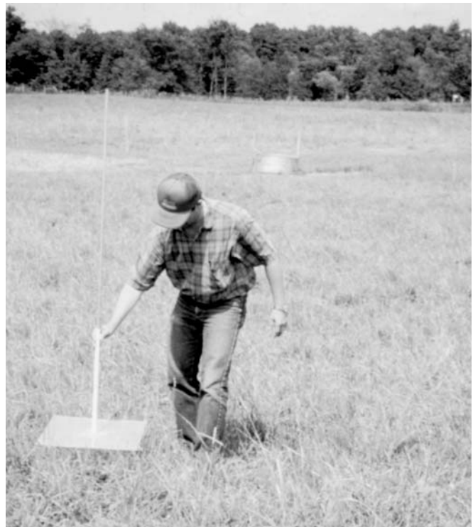
Disk or plate meters help assess the density of the pasture and improve the accuracy of pasture forage estimation over height measurements alone.
