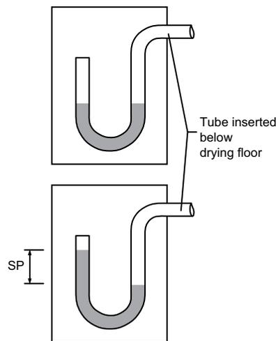
**Fig. 2. Two manometers.** The water is at the same level in both sides of the top manometer. The static pressure (SP) is zero inches, indicating the fan is not operating. When the fan is operating, as indicated in the bottom manometer, the water is pushed down in the right side and up in the left side. The distance SP between the two water levels is the static pressure measured in inches.
