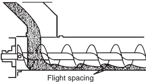
Figure 7. Feed flow in feeder.
