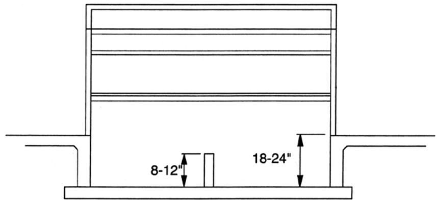
**Figure 6. Gutter under raised decks.**
