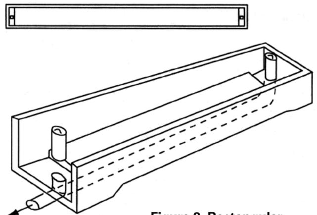
**Figure 2. Rectangular gutter with a step down.**
