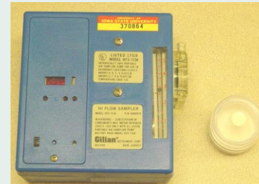
Figure 9. Filtration pump and filter
