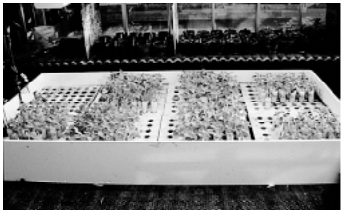
Soybean seedlings growing in temperature-controlled water bath used to conduct the follow-up greenhouse test of soil samples with low SCN egg counts.
