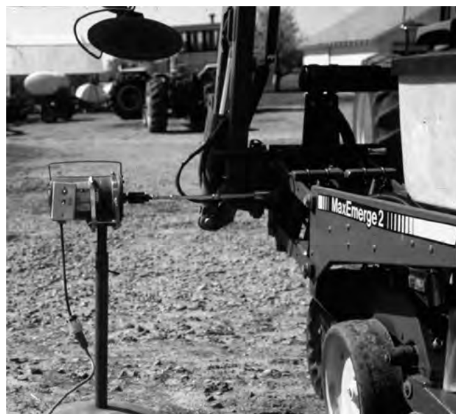
An electric calibration motor attaches onto the drive shaft of a planter with conventional 3/8" drive sockets.
